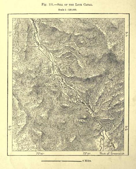
the valleys of the Chagres on the Atlantic and of the Rio Grande on the Pacific side. The crest of the range was to be crossed at Mount Culebra, either by a tunnel 130 feet high or by a tremendous open cutting. Reservoirs were to be constructed by means of dams to control the flood waters of the Chagres and its affluents, the displacement of matter being estimated at first at 1,645 millions of cubic feet, and afterwards at 2,520 millions, to allow for a tunnel nearly four miles long. But the
