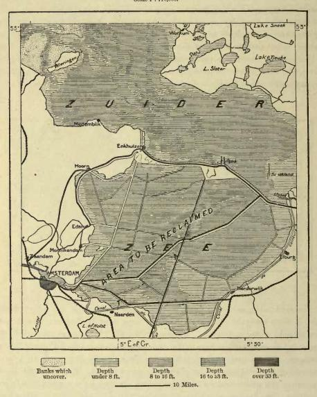
Fig. 263.—The Proposed Drainage of the Zuider Zee.
