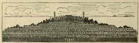
Fig. 281.—Section of the Pier Head at Ymuiden.
