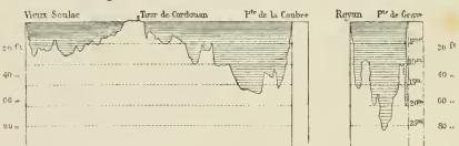
Fig. 37.—Section of the Passes of the Gironde.
