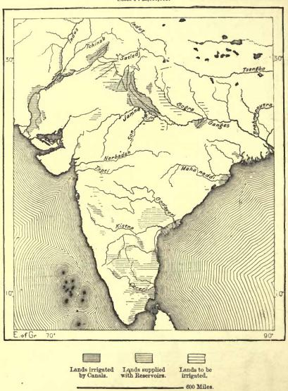
Fig. 175.—IRRIGATION WORKS OF INDIA. Scale 1: 25,000,000.
