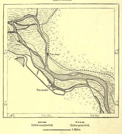
Fig. 215.—Dykes of the Irrawaddi at Henzada. Scale 1: 200,000.
