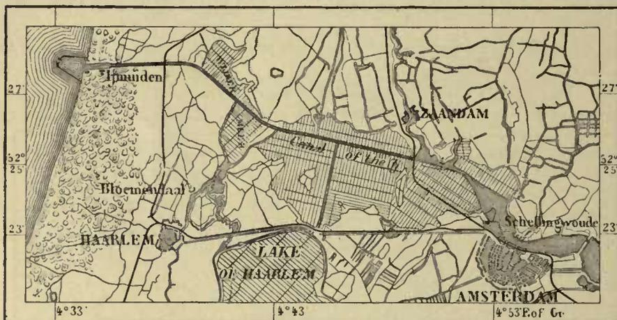
fore, to construct a new canal, the engineers naturally choosing the narrow neck of land known as *Holland op zijn smalst*. This canal of the Y, constructed since 1858, has a length of 25,886 yards, and is 207 feet in width. Its depth, as far as the great flood-gate at Ymuiden, is only 13 feet, but beyond it deepens to 25 feet. The harbour at Ymuiden is formed by two piers, each 5,000 feet in length, and covers an area of 297 acres. The entire work cost nearly
