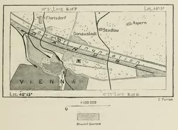
Fig. 23 .- The Rectification of the Danube at Vienna.
